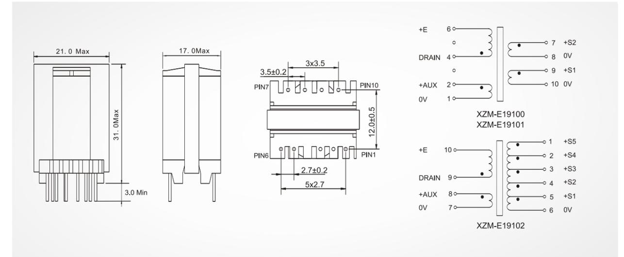
PCB Hole Diameter = 1.1mm
