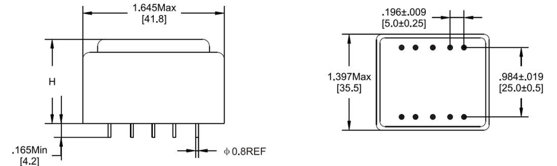
Recommended Drill Hole Diameter for Pins  $\frac{0.051 \text{ inches}}{1.30 \text{ mm}}$
