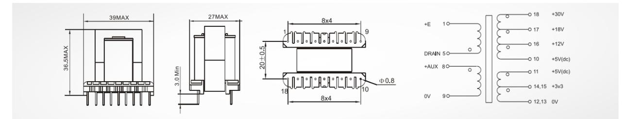
PCB Hole Diameter=1.3mm
