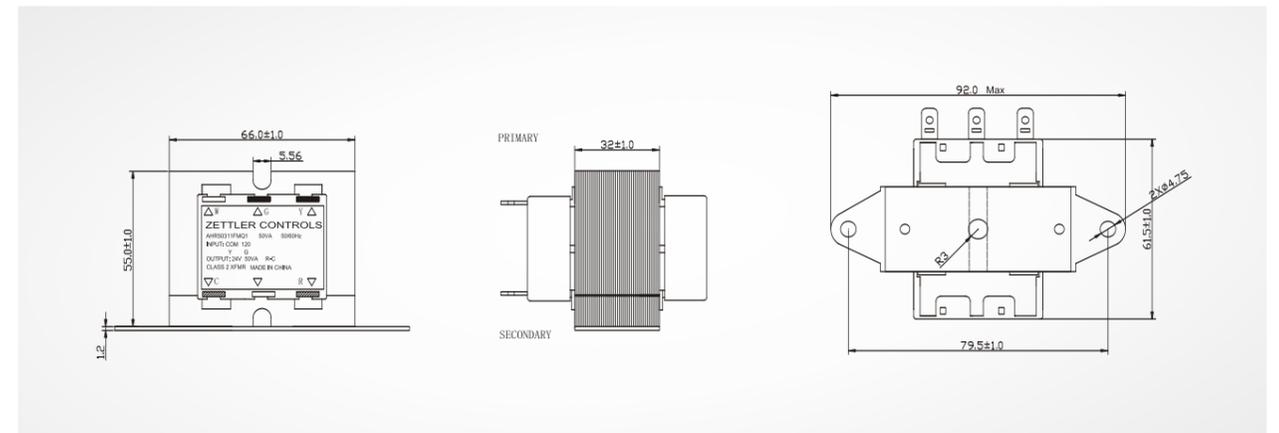
TYPE FMQT FOOT MOUNT BRACKETS WITH TOP MOUNTED QD TERMINALS
