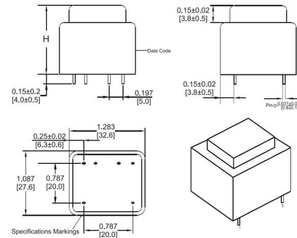
Recommended Drill Hole Diameter for Pins 0.051 inches / 1.30mm
