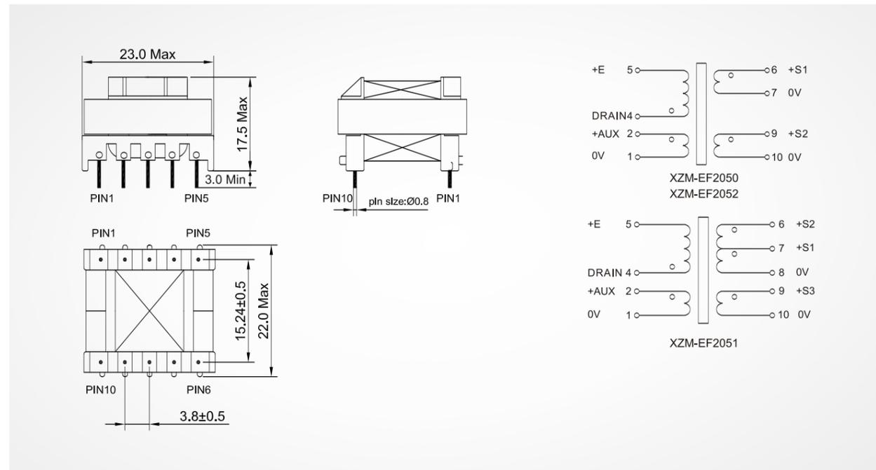
PCB Hole Diameter=1.2mm
