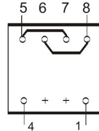
Recommended layout for transformers with 1 Secondary winding (allows the use of a transformer with 2 secondary windings)
