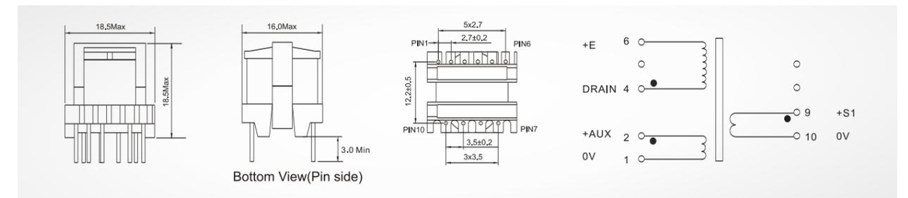
PIN 3 Removed PCB Hole Diameter = 1.1mm
