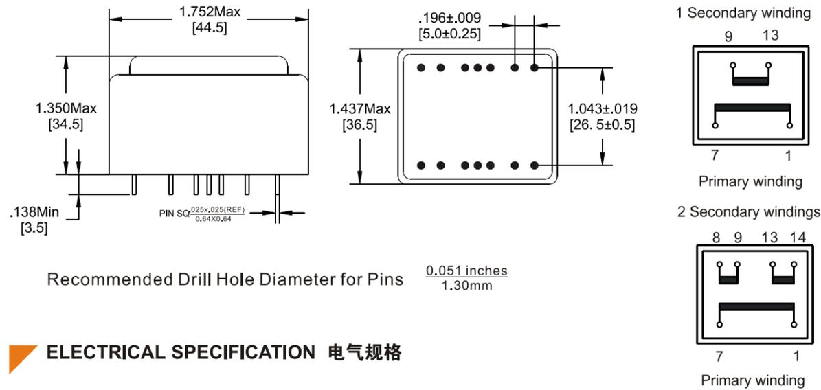
Recommended Drill Hole Diameter for Pins  $\frac{0.051 \text{ inches}}{1.30 \text{ mm}}$
