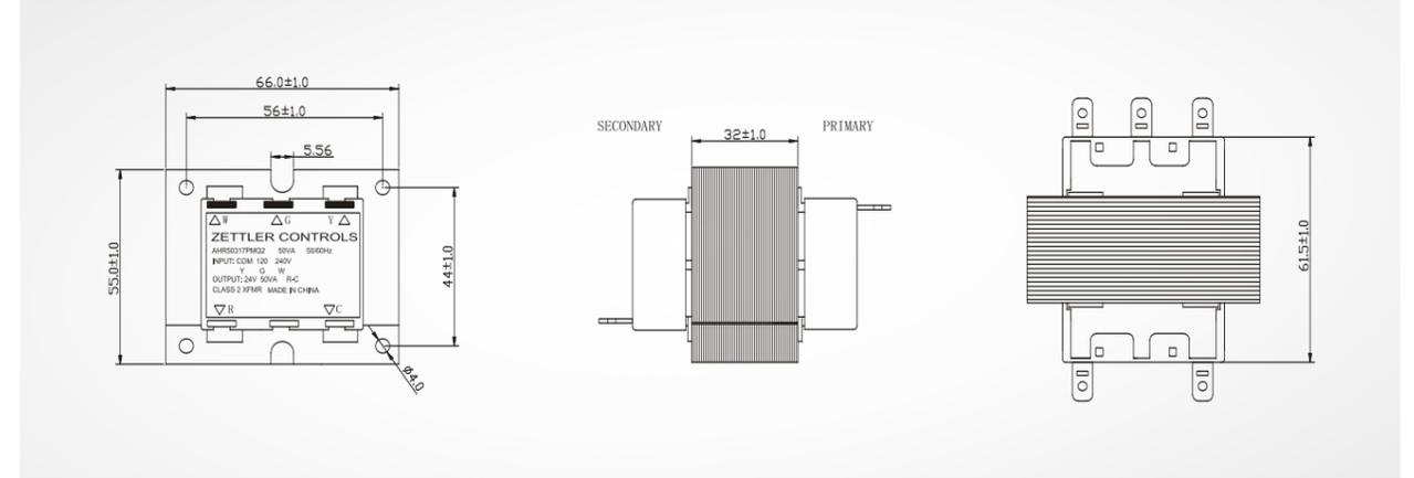
TYPE FMQW FOOT MOUNT BRACKETS WITH QD TERMINALS AND WIRE LEADS
