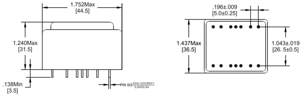
Recommended Drill Hole Diameter for Pins  $\frac{0.051 \text{ inches}}{1.30 \text{ mm}}$
