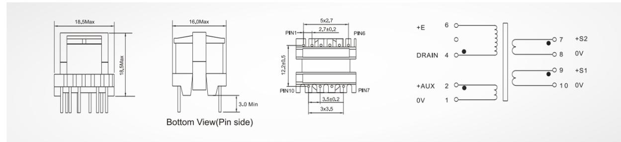
PIN 3 Removed PCB Hole Diameter = 1.1mm
