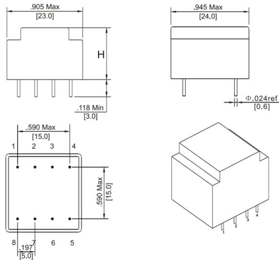
Recommended Drill Hole Diameter for Pins  $\frac{0.039 \text{ inches}}{1.0 \text{ mm}}$
