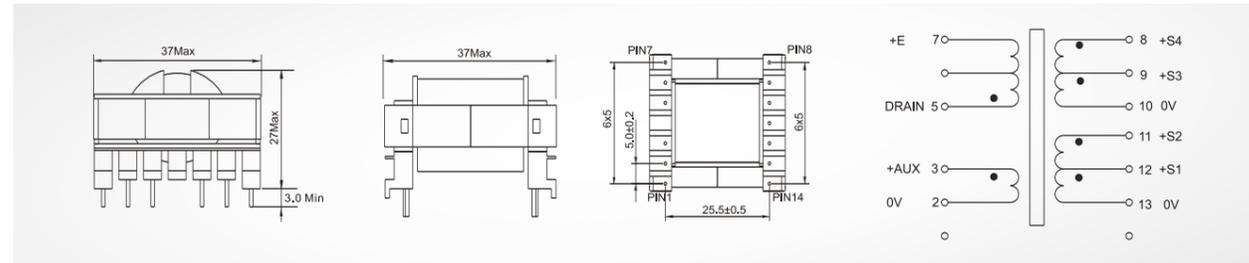
PIN 4 Removed PCB Hole Diameter=1.3mm
